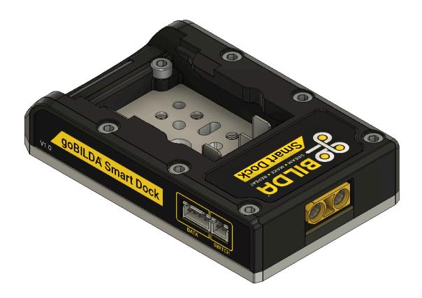
**Protection/Battery Management Features:** The Smart Dock has 3 protection features to prevent damage to the battery and the devices it powers. If any of these protection features are activated, power to the XT90 connector will be disconnected. The Smart Dock must be power-cycled by turning the switch off and on before power can be output via the XT90 connector.
