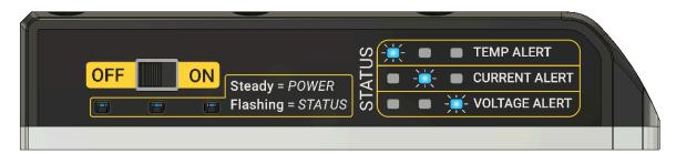
**Status LEDs:** There are 3 LEDs that describe the state of the Smart Dock. These LEDs are located directly below the power switch. When no protection feature is active, the status LEDs indicate the battery level. 3 solid LEDs indicate full charge, 2 solid LEDs indicate half charge, and 1 solid LED indicates a low battery (you may continue to use the battery with 1 solid LED, as the Smart Dock will cut off power at a safe minimum voltage).
