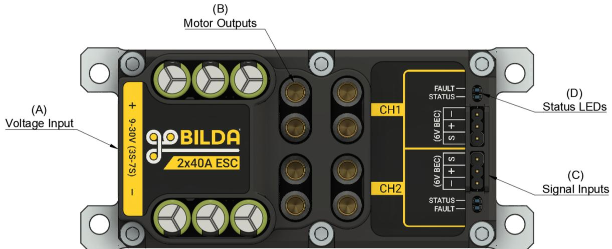
**(A) Voltage Input:** The ESC requires a DC input voltage between 9 and 30V. Choose a voltage that is appropriate for the motors you plan to use with the controller. The power input port is an XT90 connector that supplies power to both channels. This power input is reverse-polarity protected up to -30V.
