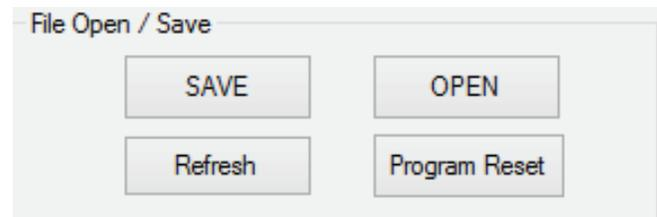
Once you have completed your servo setup and written the setup to the servo click on “SAVE” to open the save file dialog box. Navigate to the location where you want to save your file. Enter a name for your servo and click “Save.” You have successfully saved your servo parameters to a file.
