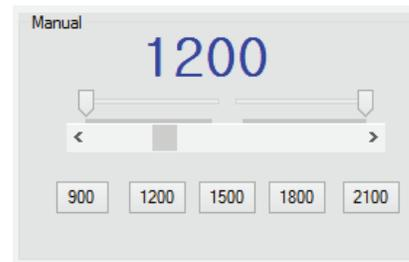
Once you have your desired Fail Safe position, click on the “FS-Position” button Fail Safe Test as seen in the illustration.
