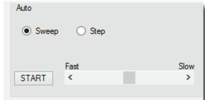
1. Select Step and click the START button. Your servo will start moving from end point to end point in a series of small “steps”.
