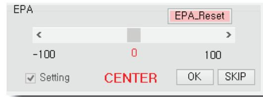
The first setting is the center point, click "OK" to continue. You can adjust the center point using three different methods.
