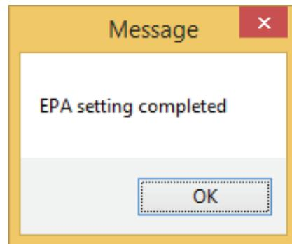
To reset your EPAs to the factory defaults, click on the "Setting" box under the EPA programming section then click EPA Reset. A message will appear indicating the reset was successful.
