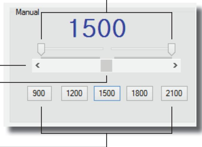
**⚠NOTE** - You can use the Endpoint Slide Bars bar to set the end points for both auto sweep and auto step functions as described below
