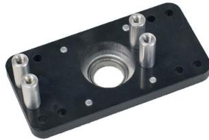
**2.** Attach the (4) .625" Length Aluminum Standoffs to the smooth side of the ABS plate using (4) 6-32 x 3/8" Pan Head Phillips Screws.
