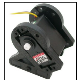
8. Press the servo plate onto the bottom plate and screw together with (1) black #4x1/2" Phillips Pan Head Screw.
