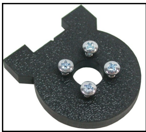
1. Install (4) 6-32 x 3/8" Pan Head Machine Screws through the holes on the textured side of part shown in the picture above.
