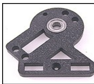
3. Install the 1/4" bore ball bearing on the textured side of the part in the picture above. The bearing may need to be lightly tapped in place with a hammer.
