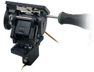
**20.** Next, tighten the top servo mounting screws.
