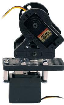
**10.** Press the servo plate onto the tilt base plate and screw together with (1) black #4x1/2" Pan Head
