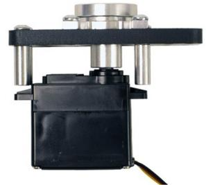
4. Put the servo onto the Servo Shaft Hub. If your servo has Karbonite gears the fitment may be very tight. Once you get it started, you can pull the horn onto the servo by installing and tightening down the stock servo screw in step 5.
