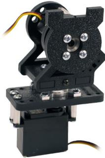
**14.** Plug the tilt servo into your servo controller and install the plate onto the servo using the factory servo screw. Operate the servo to view tilt range and adjust as needed.
