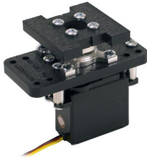
6. Plug the pan servo into your servo controller and set the controller to the neutral position. Connect the tilt base plate to the top of the Servo Shaft Hub using (4) 6-32 x 3/8" Pan Head Phillips screws. Rotate with controller to confirm the proper position of the tilt base plate at this time as it is difficult to re-index after this step.
