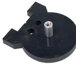
**15.** Using a 6-32x3/8" Pan Head Phillips Screw, attach the .5" length aluminum standoff to the smooth side of the part above.
