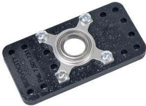
1. Attach the 1/2" Bore Flat Bearing Mount to the rough side of the ABS plate with (4) 6-32 x 3/8" Pan Head Phillips Screws.
