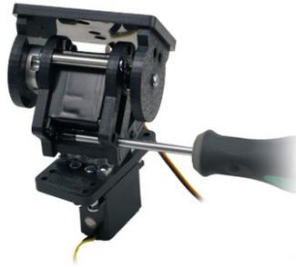
**19.** Raise or lower the servo to make the top plate level. Once level, tighten the bottom servo mounting screws.
