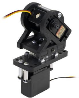
**11.** Install the 1.25" length aluminum standoff as shown above using (2) 6-32x3/8" Pan Head Phillips Screws.
