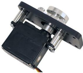
5. Attach the servo to the .625" Standoffs using (4) 6-32 x 3/8" Pan Head Phillips Screws. Make sure to install all 4 screws prior to tightening down for proper alignment. Next, install the stock servo screw into the servo to hold the Servo Shaft Hub on.
