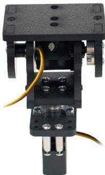
**18.** Slide the top plate in place. If the side plates are too far apart, remove spacers as necessary. Install (2) #4 x 1/2" Flat Head Phillips Screws to hold top plate on.
