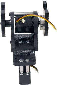
**17.** With the spacer(s) installed insert the standoff into the 1/4" flanged bearing as shown above.
