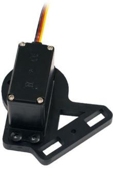
**9.** Install your tilt servo on the smooth side of the servo plate using (4) black #4x3/8" Truss screws. **Do not fully tighten!**
