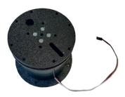
8. Using a #2 Phillips Screwdriver and (4) M4 x 12mm Zinc-Plated Flat Head Screws, attach the ABS Top Plate to the threaded holes of the Servo Hub-Shaft. If you wish to attach a camera, tilt system or goBILDA® component to the top of the pan system, you can leave this plate off and fasten the item directly onto the Hub-Shaft using appropriate M4 screws.
