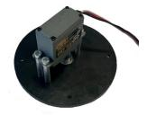
4. Using a 3mm Hex Key and (4) M4 x 10mm Zinc-Plated Socket Head Screws, attach the servo to the bottom of the Aluminum Standoffs. Make sure to start all 4 screws prior to tightening down any of the screws to allow proper alignment between the servo and the Hub-Shaft.
