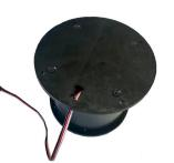
6. Using a #1 Phillips Screwdriver and (4) #4 x 1/2" Black Flat Head Screws, fasten the ABS Plastic Bottom Plate to the Tube. Make sure the servo wire is aligned with the cut-out to keep from pinching it during assembly.
