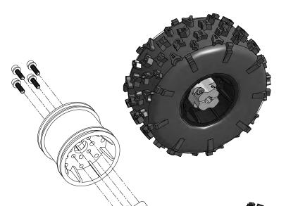
Use four 14mm length screws (each with a washer) to fasten a Hyper Hub to one of the Hurricane Wheels. Ensure the hub is on the more shallow side of the wheel. Then add a tire to the wheel.
