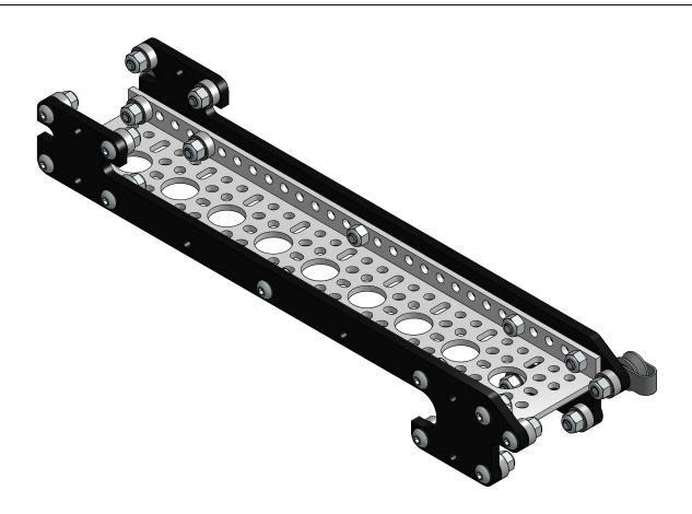
Using the last 9-hole channel, attach the bearings and stop plates as shown below. This assembly will be the second and final stage.
