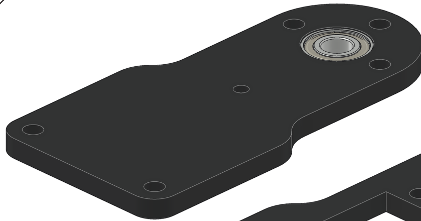
Top Plate QTY: 1 (w/ Bearing Installed)
