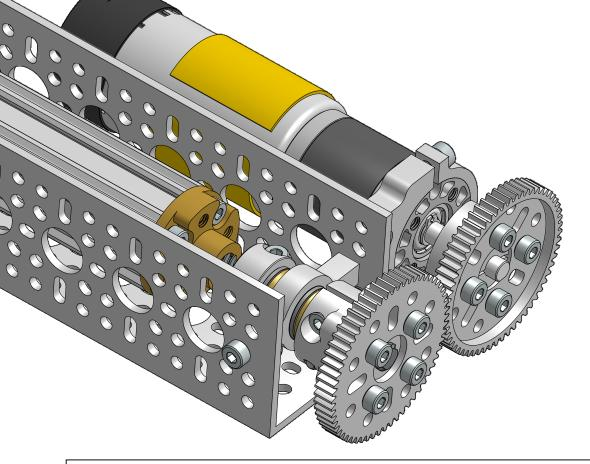
Position the gear assemblies on the motor shaft and lead screw. Slide the collar and gear on the lead screw together towards the pillow block. Tighten the pinch bolts on the collar and both hubs.
