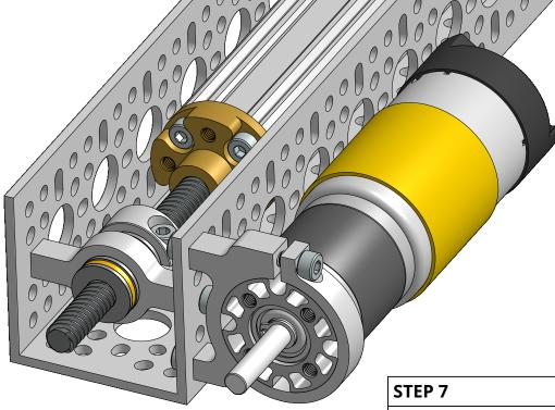
Insert a motor into the clamping mount as shown. Tighten the pinch bolt. This kit does not include a motor; a 5202-0002-0005 is shown as an example.
