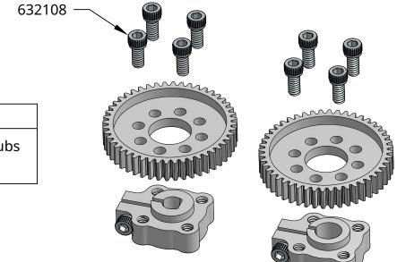
Fasten the gears to the hubs using eight 5/16" screws.
