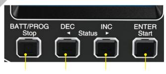
BATT. Type/Stop Button Stop the progress of the current action or cycle back to the previous step / screen. DEC. Button Scroll through available menus or decrease parameter values. INC. Button Scroll through available menus or increase parameter values.
