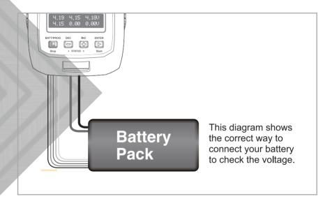
BATT/PROGRAM BATT METER Press the START/ENTER button to access the Lithium Battery Meter program.
