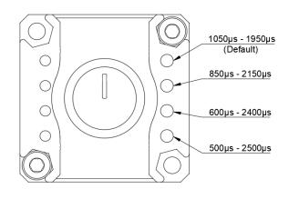
**1050µs-1950µs** is the default PWM range. This range allows most servos to rotate 90 degrees. Many servos are able to rotate further, given a wider range. If you purchased a goBILDA® Servo, reference the servo page for the maximum PWM range the servo is able to accept, and the corresponding rotation. This range is also used with goBILDA linear servos.
